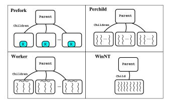
Figure 1: Apache 2.0 Multi-Processing Modules.
