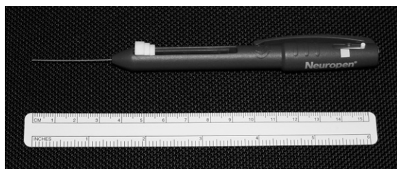
Fig. 1 The Neuropen, with the monofilament fully deployed from its distal end, shown next to a centimetre rule.
